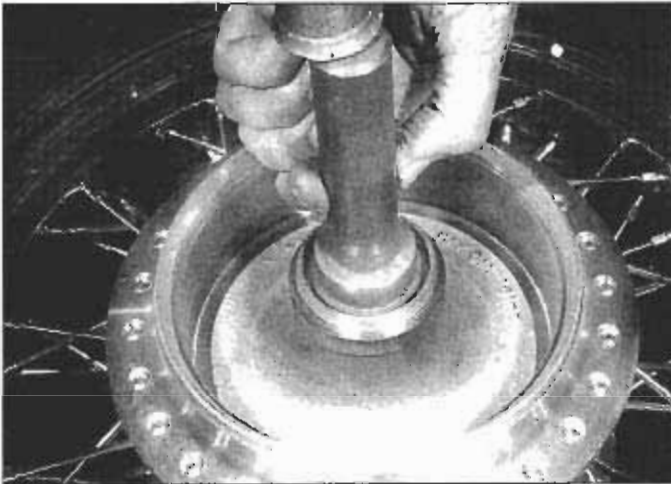
13.20c Install the new bearings with a seal driver, a large socket or a section of pipe
