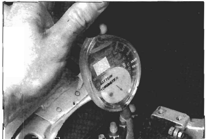
4.7 Check the specific gravity with a hydrometer
