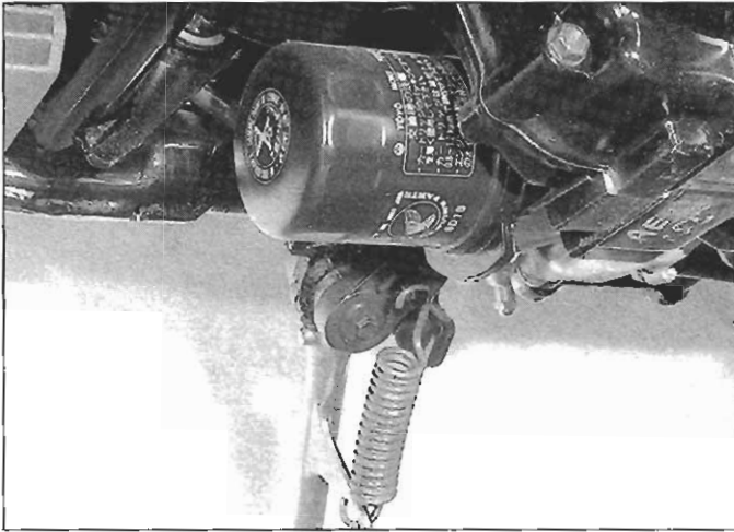
12.5a The oil filter (arrow) is at the left lower rear of the engine; the easiest way to reach it is from the right side, with the bike leaned over to the left on its sidestand
