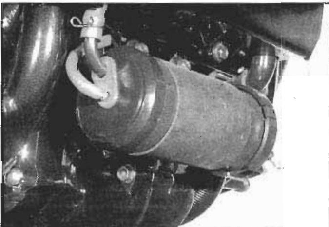
5.1 The EVAP canister is located below the radiator; make sure that all hoses are in good condition and are securely attached to the canister
