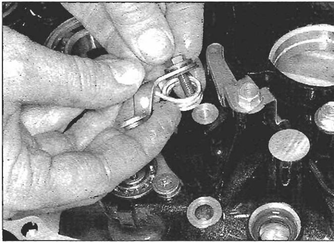
22.14 Remove the stopper arm bolt, washers, stopper arm and return spring
