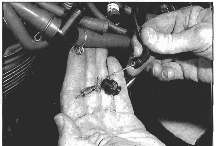
9.15 Before adjusting the choke cable, inspect the spring, valve and threaded barrel of each SE valve; replace any broken or worn pieces
