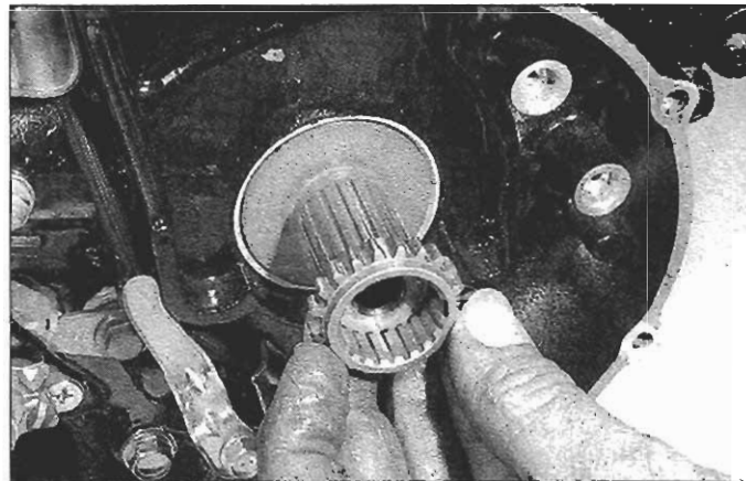
21.12b The drive sprocket for the rear cylinder crankshaft cam chain is removable; if it's worn or damaged, replace it
