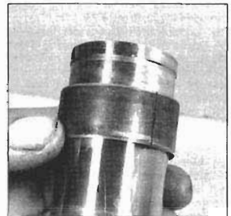
5.11c . . . the slider bushing can now be removed by sliding it off
