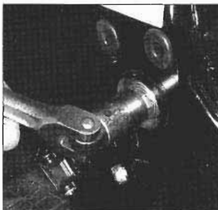
10.8c Use a 17 mm Allen bolt bit in a socket to hold the right pivot bolt while you turn the locknut, and to unscrew both pivot bolts
