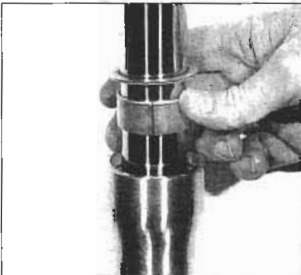
5.23 Install the back-up ring on the fork tube
