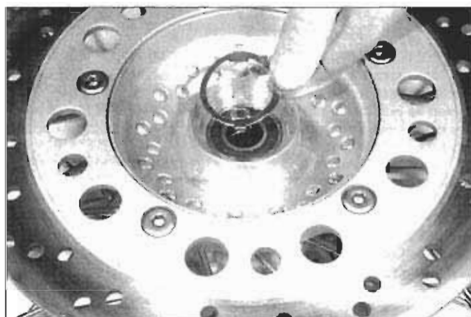
13.3b Remove the retainer for the speedometer gearbox unit
