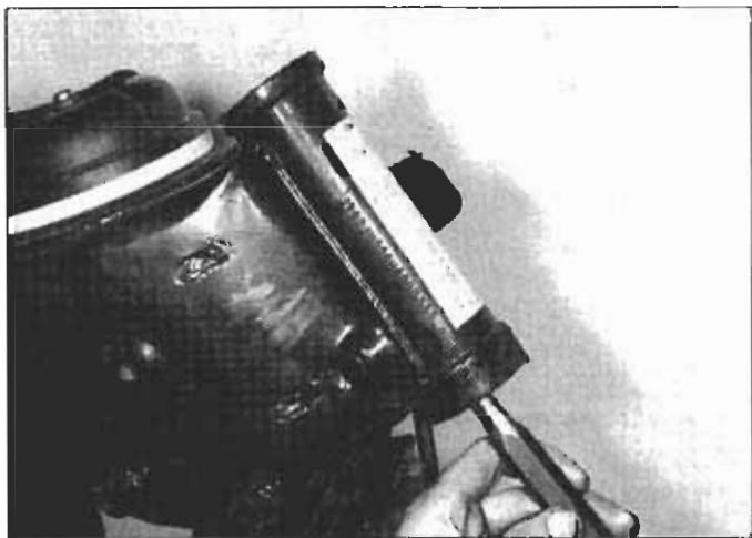
6.12a Insert a long punch or rod from below to tap out the upper bearing outer race . . .
