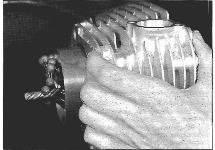
14.14 Move the hone rapidly up-and-down without stopping
