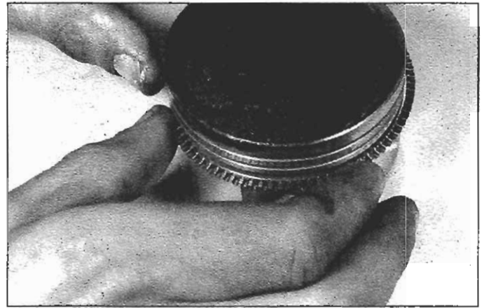
16.9a Install the oil ring expander first
