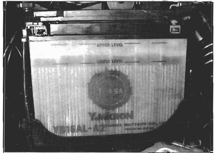
4.4 The electrolyte level should be between the marks on the battery case
