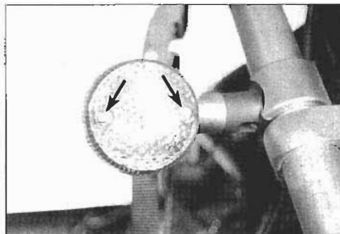
10.1 To detach a turn signal lens, remove these two retaining screws (arrows)
