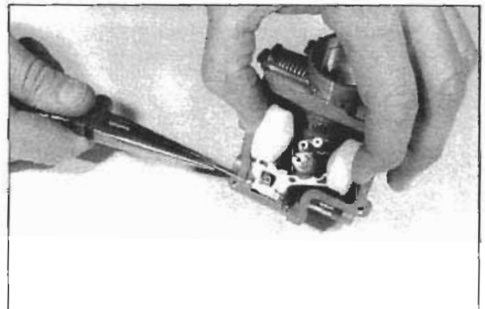
13.8 Unscrew the float valve seat (1), the main jet (2) and the slow jet (3); don't lose the washer for the float valve seat
