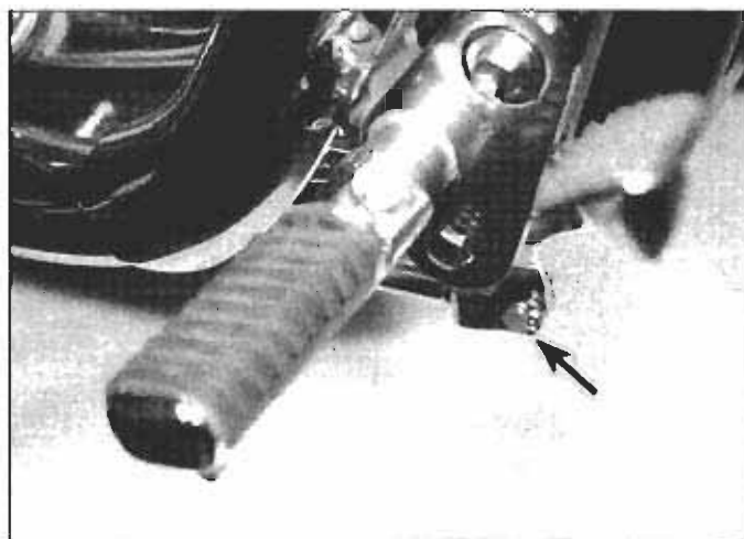
9.4a Remove the cotter pin, pull out the clevis pin (arrow) and disconnect the middle brake rod from the brake pedal arm . . .
