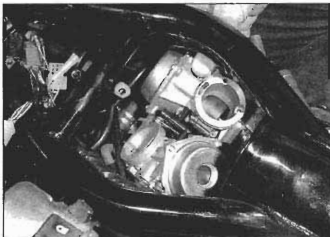
12.12c ... rotate the carburetors so that they're positioned at a 90-degree angle to their installed position ...
