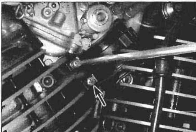
12.12a Loosen both insulator clamp screws ...
