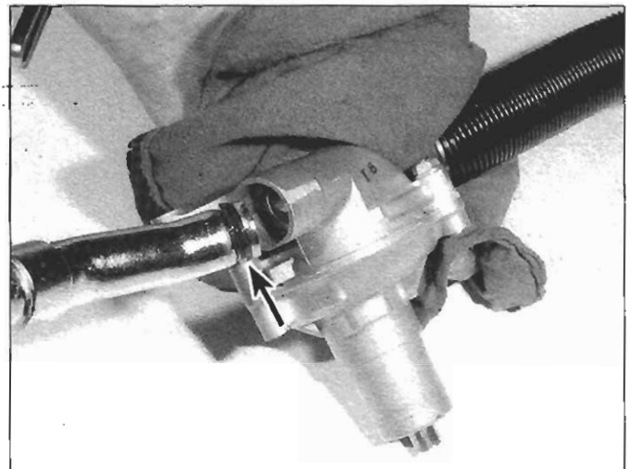
9.12 Install a new O-ring on the outlet pipe (arrow)
