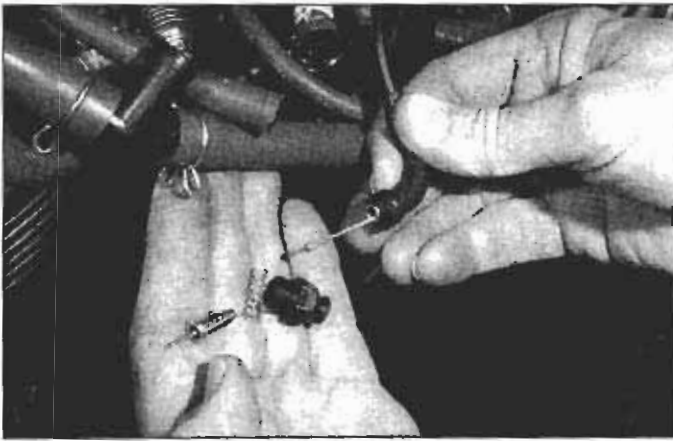
12.10b ... and separate the SE valve, spring and locknut from each cable
