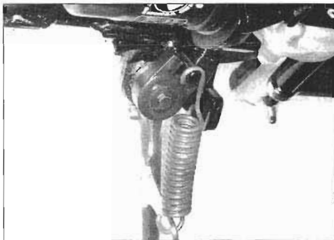
4.1 Make sure the sidestand spring is in good condition and correctly installed
