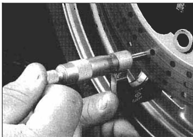
4.4a Use a micrometer to measure the thickness of the disc at several points
