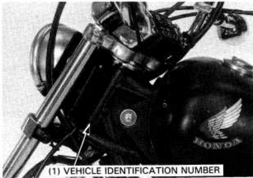
The legal vehicle identification number (VIN) is on the left side of the steering head.
