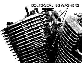
Remove the cam chain tensioner.
