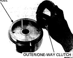
Hold the flywheel using a special tool.
