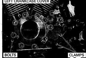
Route the wires Clamp and bind the wires with clamps and wire properly bands. (page 1-22).
