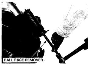
Remove the lower bearing outer race using the special tool and suitable shaft.
